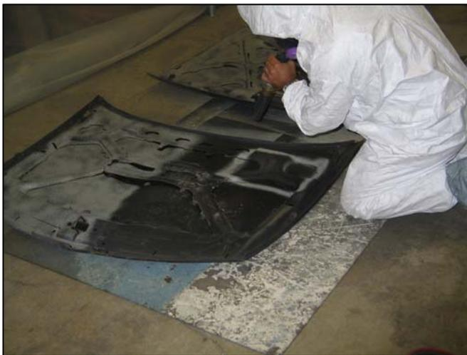
**Figure 1 - Abrasive blasting with composite abrasives during 2nd test series. Note the absence of visible airborne emissions during blasting.**
