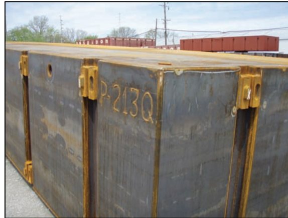
(Fig. 2) New sectional barge to be abrasive blasted
