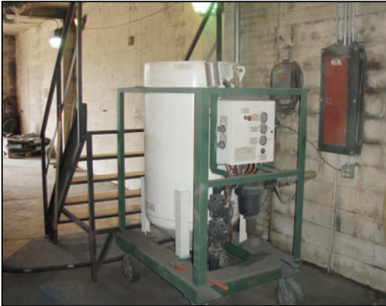
(Fig.3) 400-Liter Specialized Pressure Vessel
