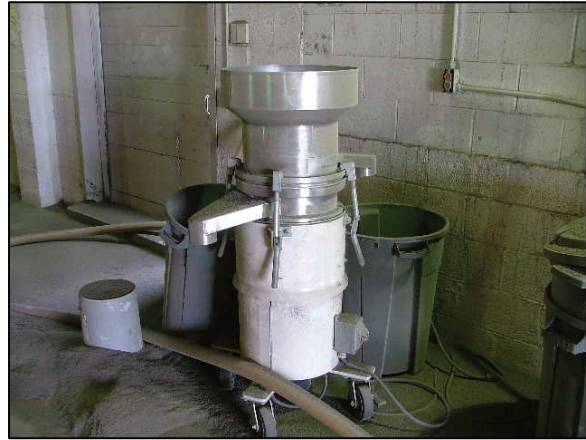
(Fig.4) Pneumatic sieve-based classifiers separate reusable media from waste
